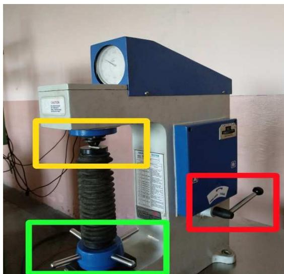
towards the top on the test table whose position has been shown by a yellow circle, the hand wheel beneath it was rotated so as to raise it to touch the indenter.
